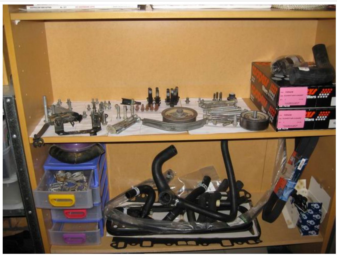
Valley Gasket – Ray from CMW advised against using the black composite one from the VRS Kit, so I got the silver (Payen) one instead.
